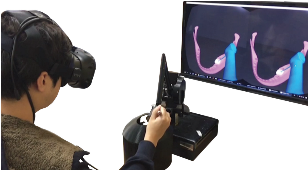
FIGURE 4.8: Virtual reality dental simulator in operation using haptic device.
