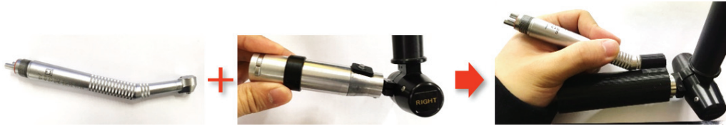
FIGURE 4.5: A dental handpiece attached to the handle of the haptic device using a 3D-printed connector.
